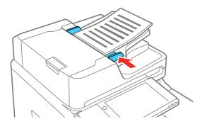
**Note:** If you are copying two originals onto one sheet, make sure the originals are loaded as shown. Select the link below to select the copy orientation setting that matches how you loaded your original.
