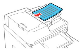
Note: Do not load originals above the arrow mark on the ADF edge guide.
