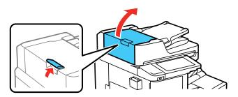
2. Use a soft, lint-free cloth (microfiber is recommended) moistened with a little water to clean the rollers and the interior of the ADF.
