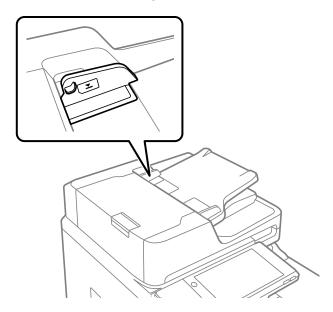
The **ADF** icon on the Copy, Scan, and Fax (models equipped with the optional fax board) screens lights up.
