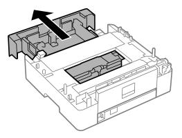
5. Slide the tab as shown and remove the back part of paper cassette 2.
